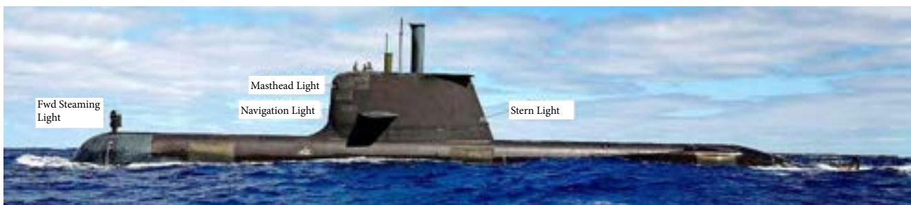
Collins Class submarine illustrating typical navigation light configuration
