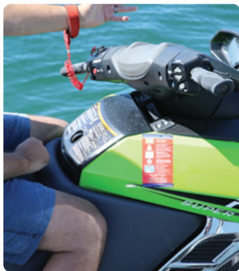
A kill switch lanyard attached to your arm stops the engine if you fall overboard.
