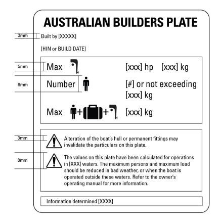
Figure A. 8—Sample ABP template for boats 6 metres or more in length, designed to be powered by an outboard engine, using text and symbols
