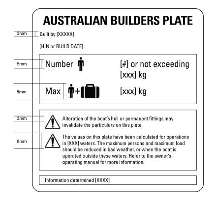
Figure A. 9—Sample ABP template for boats 6 metres or more in length, not designed to be powered by an outboard engine using text and symbols
