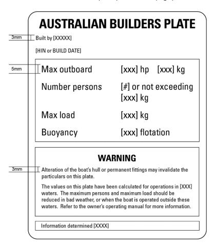
Figure A. 1—Sample ABP template for boats less than 6 metres in length designed to be powered by an outboard engine
