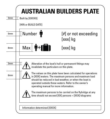
Figure A. 10—Sample ABP template for boats 6 metres or more in length and fitted with a flybridge, not designed to be powered by an outboard engine, using text and symbols
