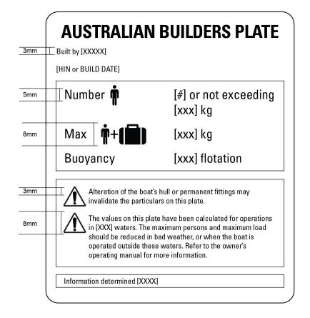
Figure A. 4—Sample ABP template for boats less than 6 metres in length, not designed to be powered by an outboard engine, using text and symbols
