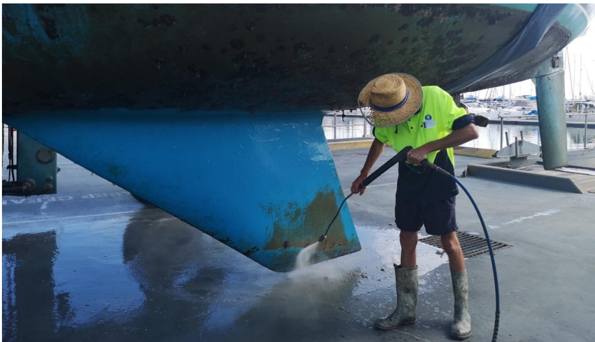
Photo 2 – Boat being cleaned and waste captured
