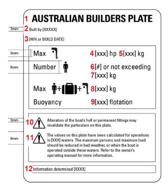
This is a sample of an ABP for a boat less than 6 meters with an outboard motor. For further details, please refer to the National Standard for Australian Builders Plate for Recreational boats.
